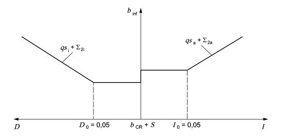
Figure 24 — Taking oscillations into account in the semi-width  $b_{inf}$
