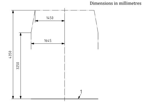
Figure C.7 shows the reference profile of kinematic gauge GB2.
