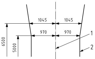
Figure G.3 — Kinematic reference profile for 25 kV pantographs in the raised position for gauges BE1, BE2 and BE3
