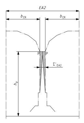
Figure I.1 — Limit distance between the track centres with allowance calculated on a straight track
