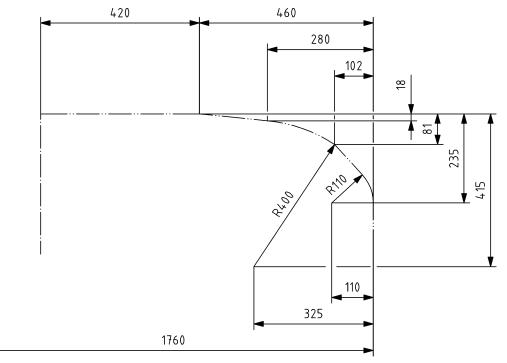
Figure G.1 — Head with 1,760 m width
