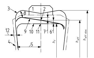
a) Pantograph fitted with insulating horns
