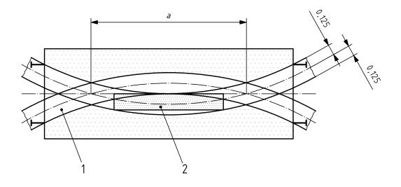
1 zone of vehicle incapable of falling more than 0,100 m from the running surface
