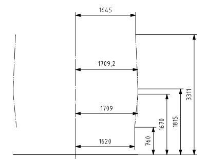
Figure C.21 — Reference profile of kinematic gauge DE1
